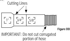
• If a longer drain hose is required, add up to 42" of length for a total of 10 ft. to the factory installed hose. Use 5/8" or 7/8" inside diameter hose and a coupler to connect the two hose ends. Secure the connection with hose clamps.
